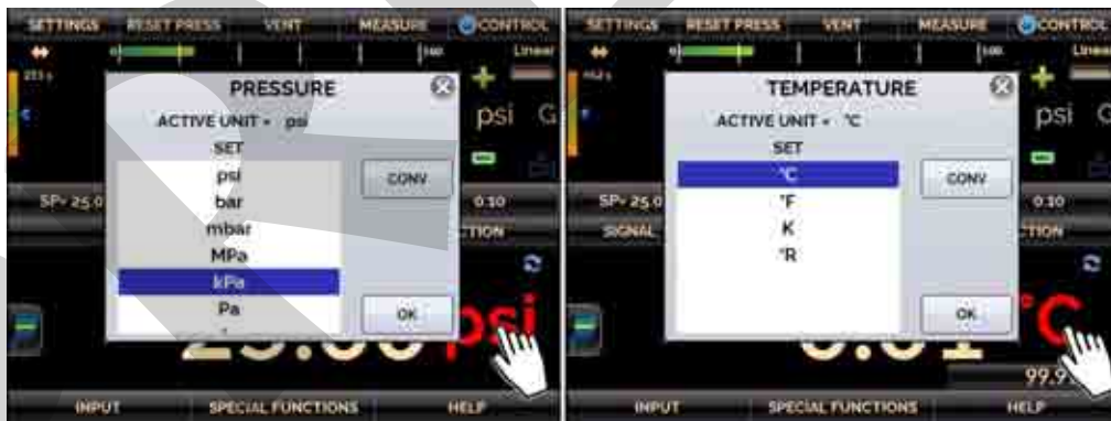
Fig. 36 - Selecting the Engineering Unit
