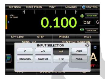
Fig. 38 – Auxiliary input type selection.
