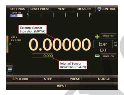
Fig. 55 - Control Mode with MPYA
