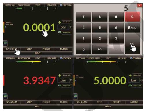
Fig. 18 – Changing the setpoint value in the CONTROL mode.
