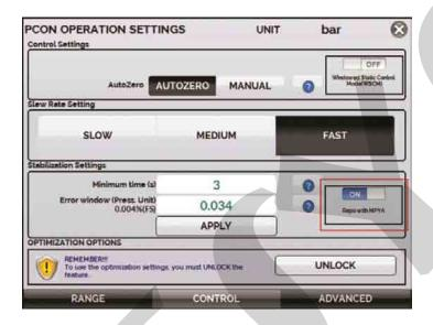
Fig. 57 - Control Mode with MPYA
