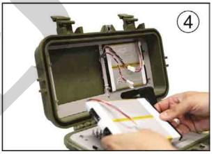
Fig. 82 - Replacing Battery Pack - FS Version over 25 bar
