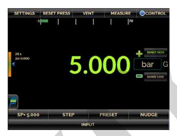
Fig. 14 – CONTROL mode on the OPERATION screen.
