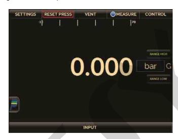
Fig. 11 – Reset pressure button on the OPERATION screen.
