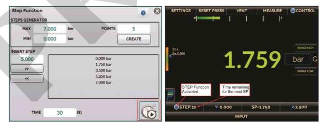
Fig. 27 – STEP Function (automatic step program).
