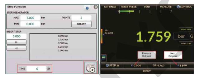
Fig. 28 – STEP Function (manual step program).
