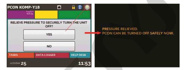
Fig. 34 – Depressurized shutdown
