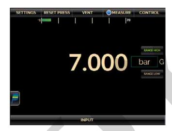
Fig. 09 – MEASURE mode on the OPERATION screen.
