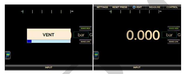
**Fig. 05** – Calibrator initialization and VENT mode on the OPERATION screen.
