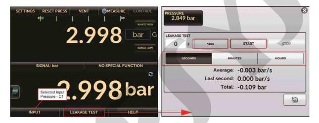
Fig. 50 – Leak test (select MEASURE mode and the Auxiliary Input).
