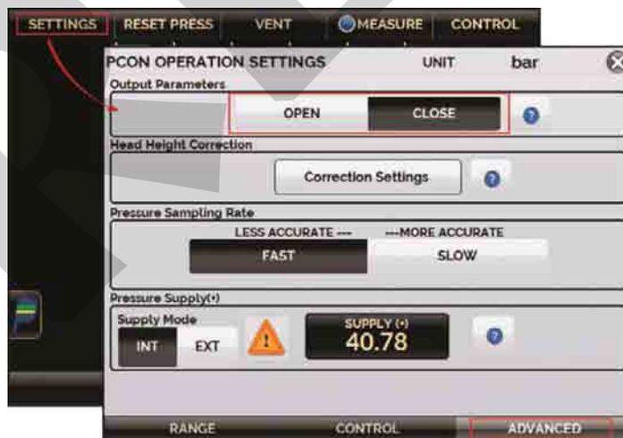
**Fig. 12** – Output Isolation Valve Status.
