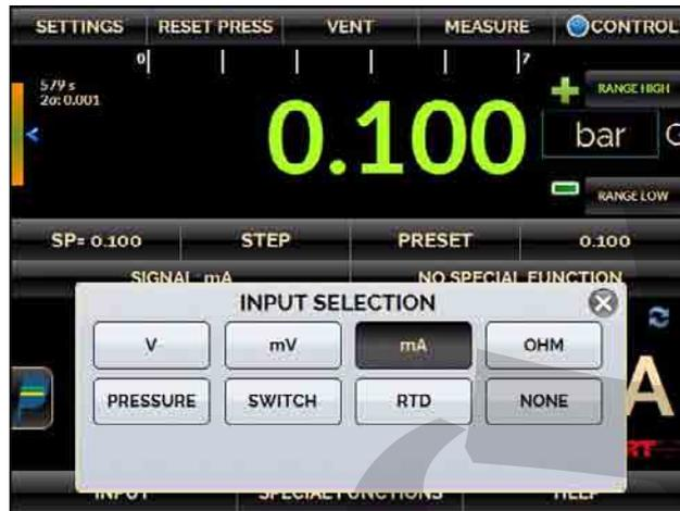
**Fig. 38** – Auxiliary input type selection.
