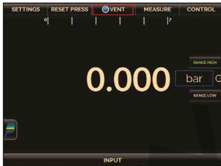
Fig. 30 – VENT mode on the OPERATION screen.
