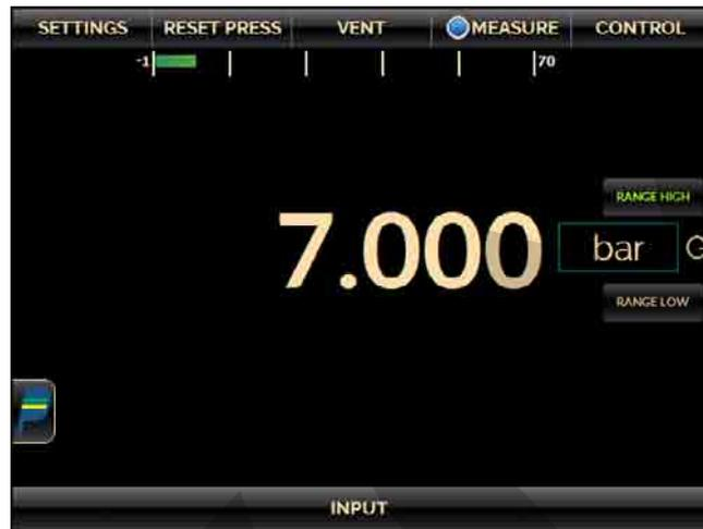
Fig. 09 – MEASURE mode on the OPERATION screen.
