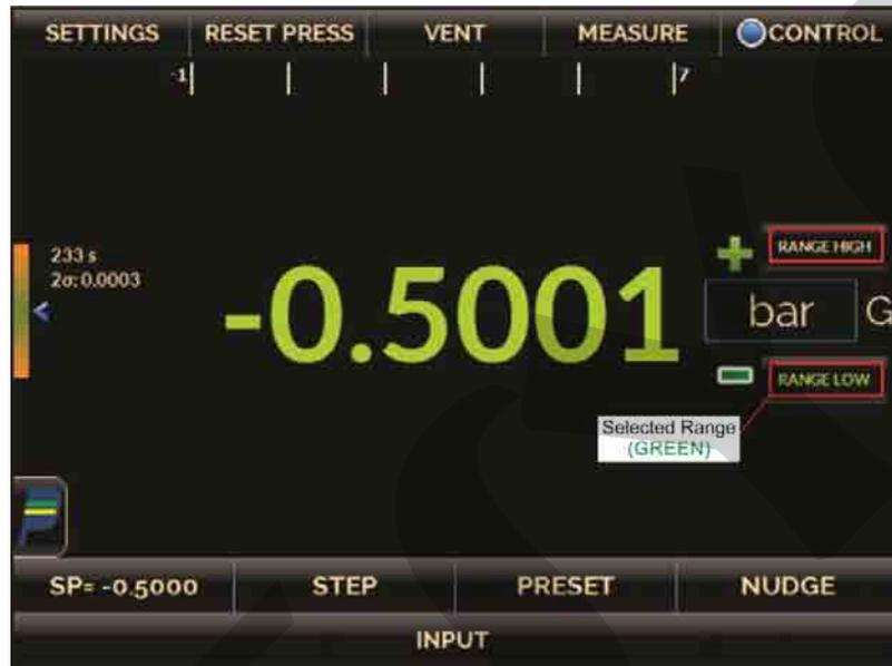
**Fig. 16** – Selecting the Pressure Range
