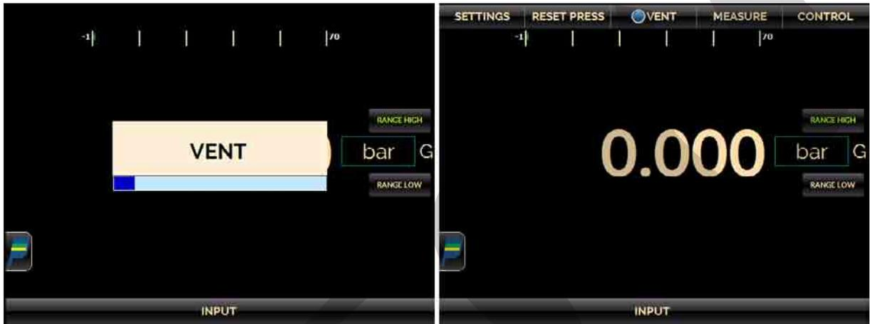
Fig. 05 – Calibrator initialization and VENT mode on the OPERATION screen.
