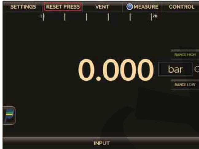
**Fig. 32** – Reset of the current pressure measurement.
