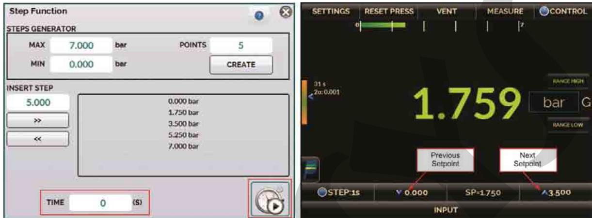
**Fig. 28** – STEP Function (manual step program).
