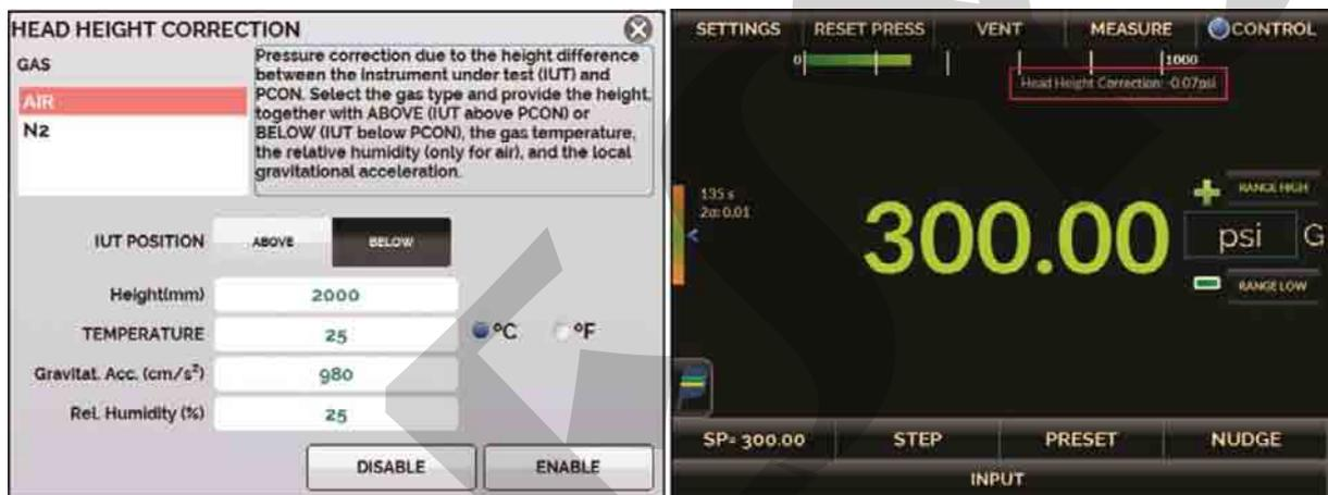
Fig. 13 – Head Height Correction
