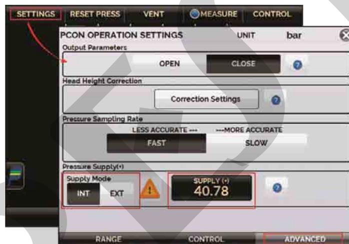
Fig. 07 – Pressure Supply Mode
