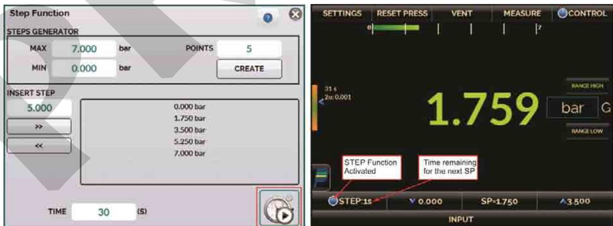
Fig. 27 – STEP Function (automatic step program).
