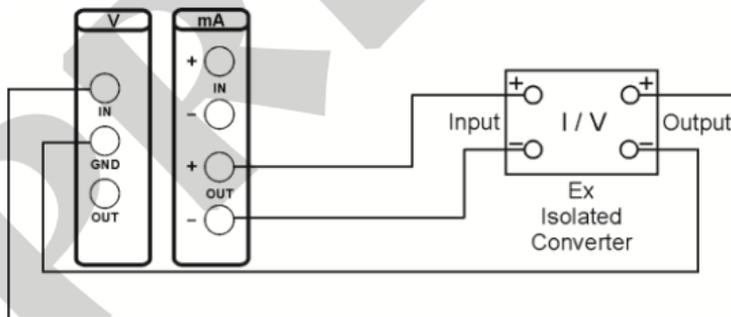
**Fig. 17 – I/V Converter (isolated)**
