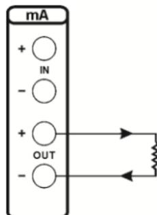
**Fig. 10** – mA Output active mode
