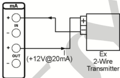
**Fig. 14 – 2-WIRE Transmitter Calibration****c) Current Supply**
