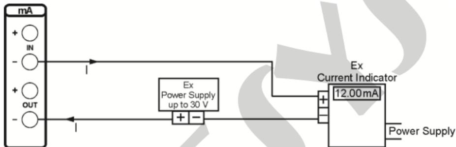
**Fig. 16 – 2-Wire Transmitter Simulation (XTR)**
