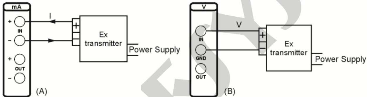
**Fig. 13** – 4-WIRE Transmitter Calibration
