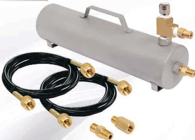
This kit is used with our pressure controllers with a negative supply (vacuum pump) to prevent positive pressure discharges from damaging the vacuum pump or reducing its efficiency when changing the setpoint.
