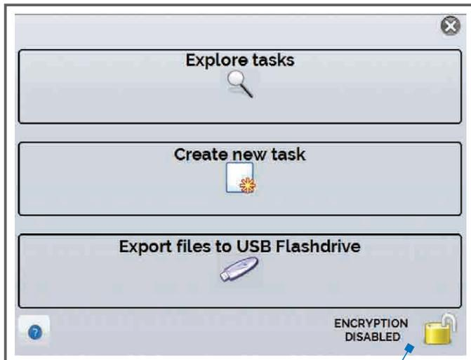
You can create tasks using the touch screen display or by connecting the PCON-Y17 to your computer. Other methods are also possible such as sending task from your application using our XML description or from an existing Excel™ application. The PCON-Y17 can also pick-up a task directly on a remote server. All these possibilities are described and documented in our communication manual.
