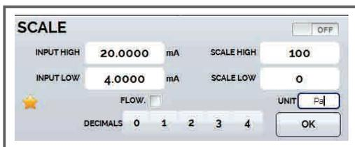
The 4-20 mA pressure transmitters can be calibrated showing directly the scaled pressure that will be displayed jointly with the measured current value.
