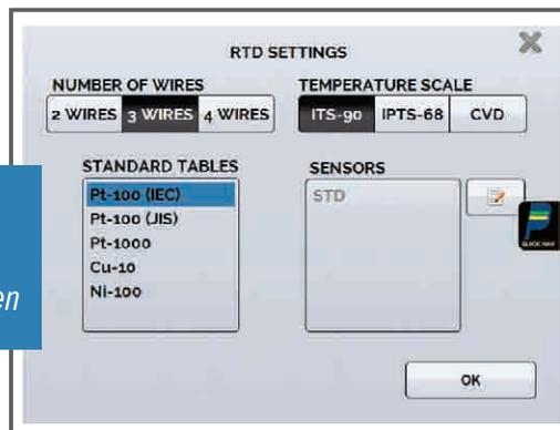
RTD can be connected with 2,4 or 4 wires and you can select various tables such as the IEC 60751, JIS or Callender-Van Dussen
