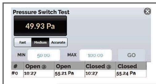
Test of your pressure switches can be performed automatically.
