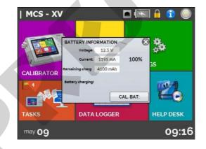
Fig. 96 - Checking battery information
