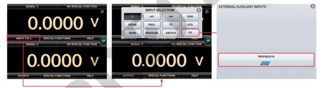
Fig. 58 - Profibus® input selection
