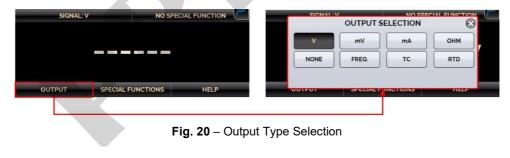
The **FREQ.** option allows the selection of the frequency or pulse generation. For the frequency generation, it must be chosen between the bands of 100 Hz or 10000 Hz. It can also be adjusted the amplitude, which varies from 0 to 22 V. For the pulse generation (square wave) in addition to the amplitude and the number of pulses, one must provide the rate at which the pulses should be sent, given in Hz. The pulse sequence is sent as soon as **OK** is pressed.
