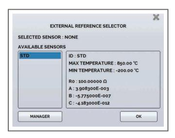
TA dry blocks are provided with an input for an external reference sensor that can be used to improve the accuracy. eliminate the offset and loading effect or work with the specific liquid stirred bath insert, black body insert or sanitary insert.
