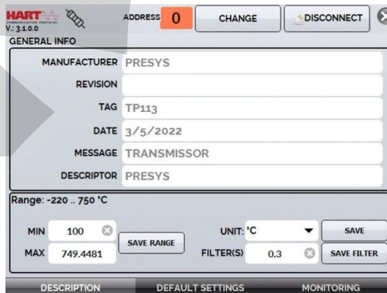
Fig. 22 - Adjusting the measuring range of the HART® transmitter
