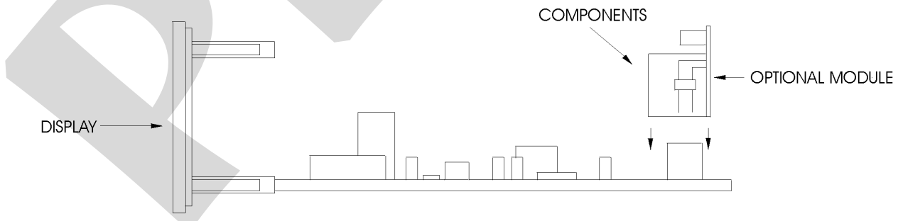
Fig. 20 - Installation of optional modules
