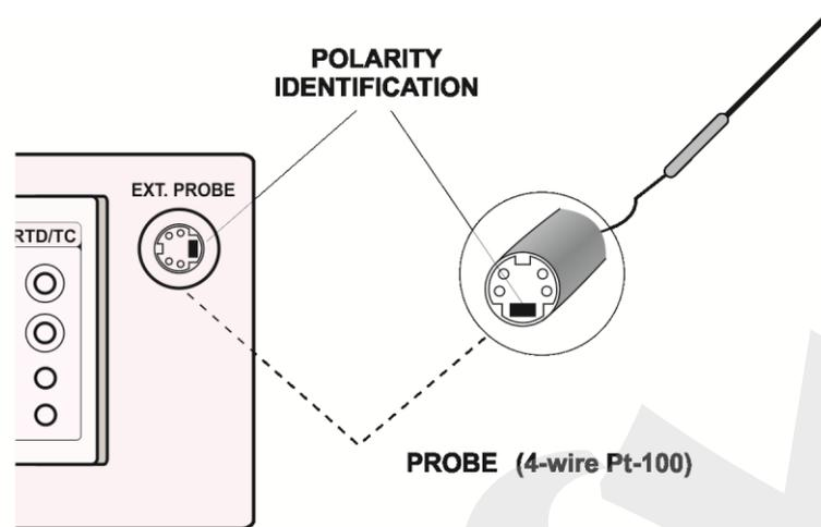
The temperature control with the external probe must be enabled by the **PRBe** option of the **PRG** menu. More details in item 2.2 - *Menu CONF*.
