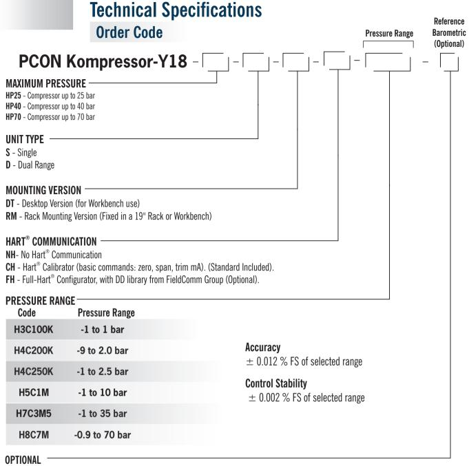
BR - Barometric Reference to measure and emulate absolute pressure Accuracy 0.16 mmHg / 0.2 mbar
