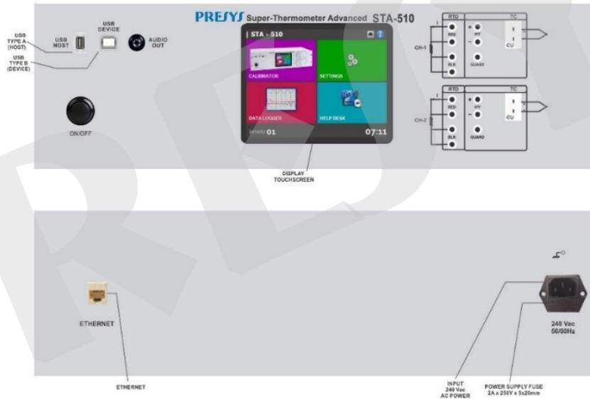
**Fig. 01 - Front and Rear Panels – STA-510-RM**
