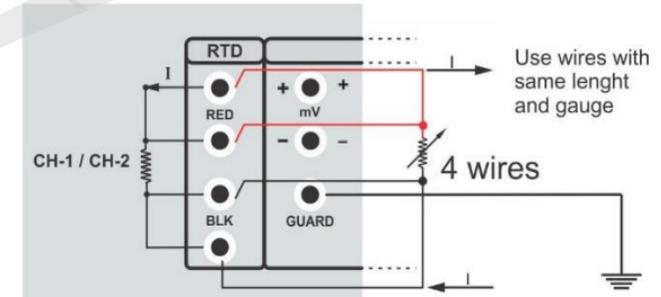
**Fig. 12 - Measurement Connections****2.3.2 - Saving Current Configuration (Memory Manager)**
