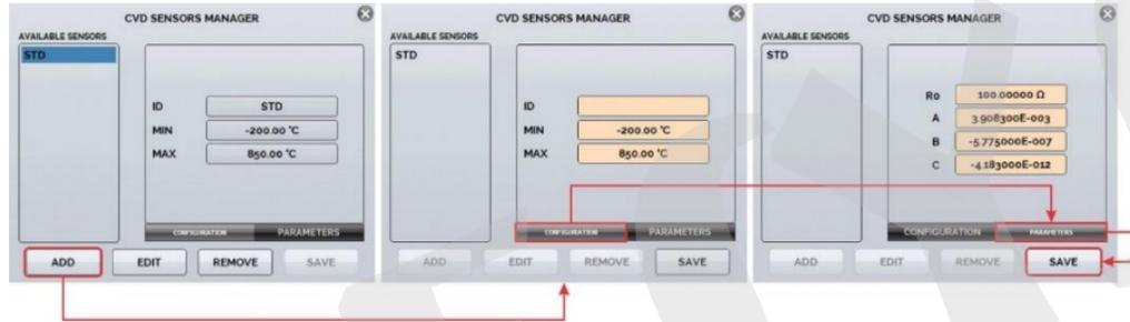
Fig. 08 - Calendar-Van Dusen Coefficient Configuration
