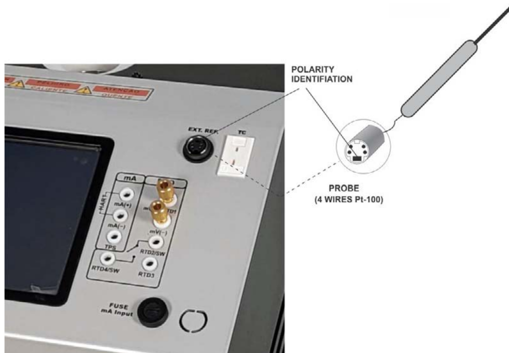
Fig. 10 - Connecting the Standard Sensor for the External Reference
