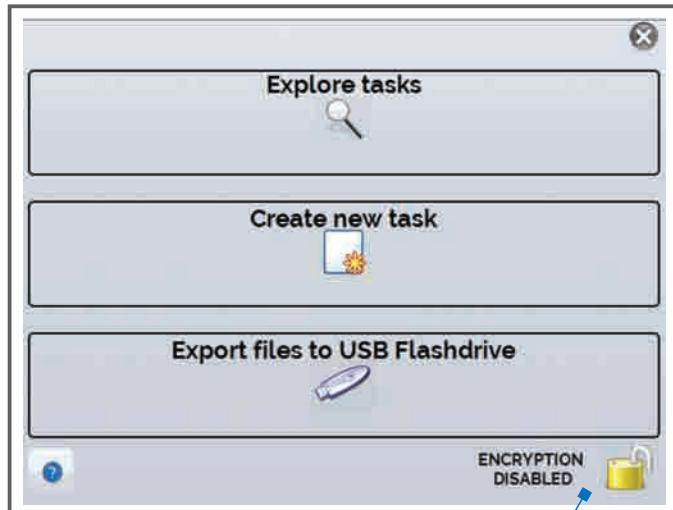
You can create tasks using the touch screen display or by connecting the PCON-Y18 to your computer. Other methods are also possible such as sending task from your application using our XML description or from an existing Excel™ application. The PCON-Y18 can also pick-up a task directly on a remote server. All these possibilities are described and documented in our communication manual.
