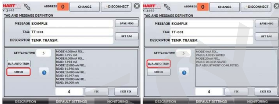
Fig. 15 - Checking / Adjusting the mA Output of the HART ® Transmitter
