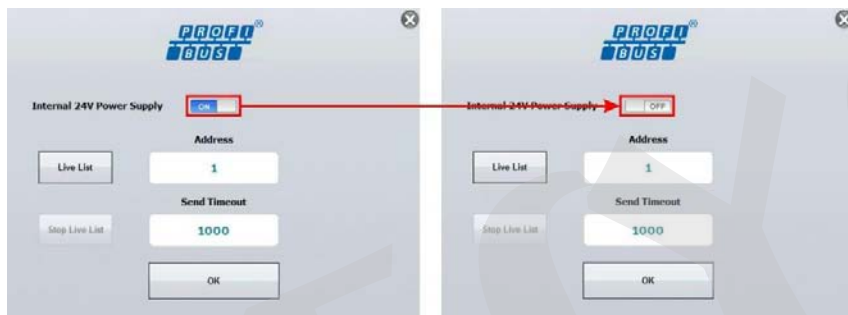
Fig. 60 - Enabling the internal power supply
