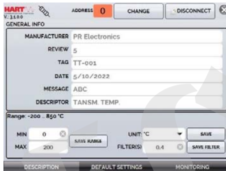
Fig. 50 Adjusting the Measuring Range of the HART ® Transmitter with Reference
