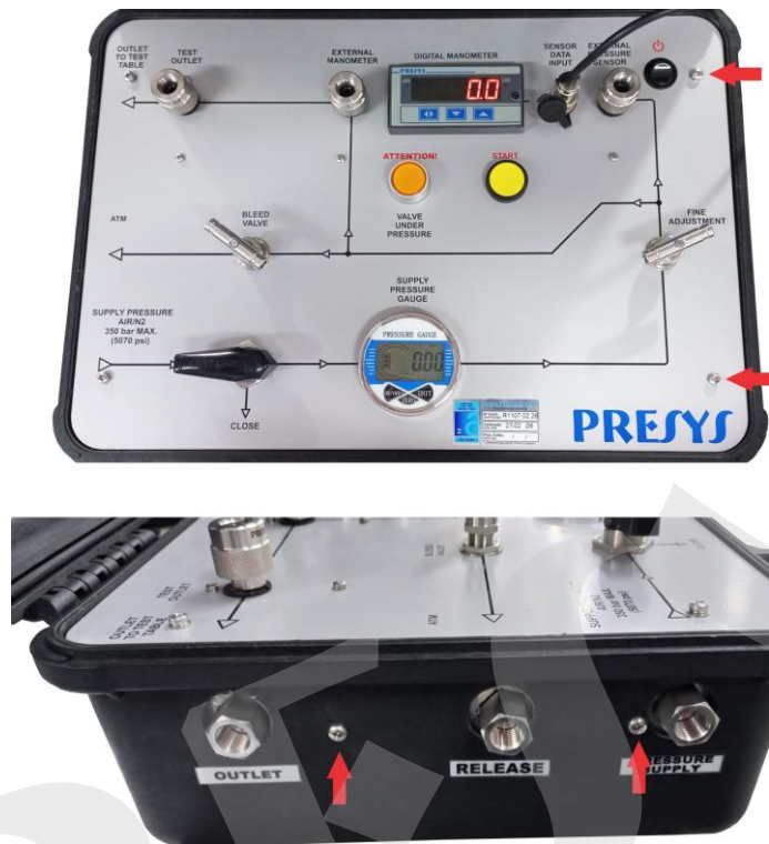
Fig. 34 - Removal of the four M4 screws
