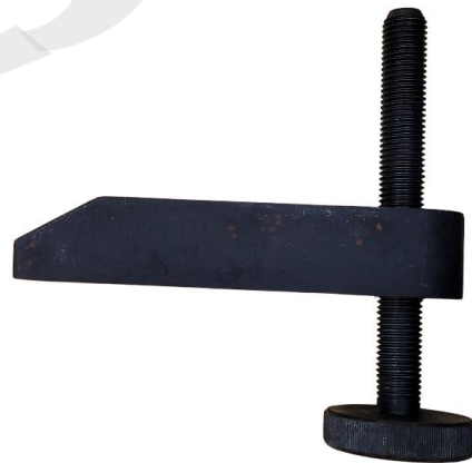
Fig. 13 - Fixing clamp and support screw
