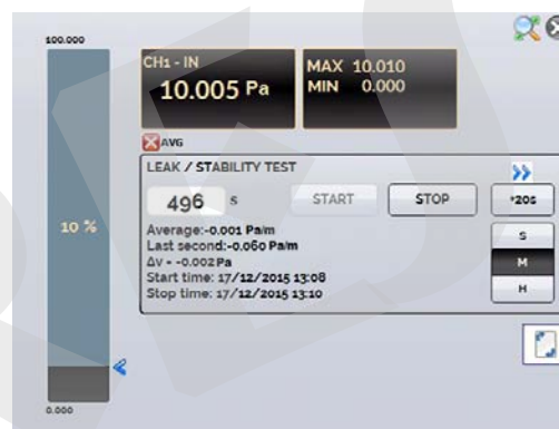
Fig. 50 - Leak/Stability Test - results
