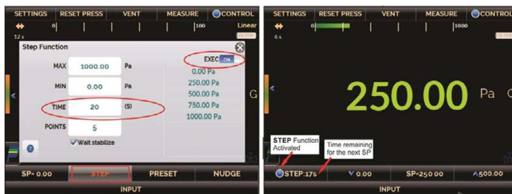
Fig. 23 - STEP Function (automatic step program)
