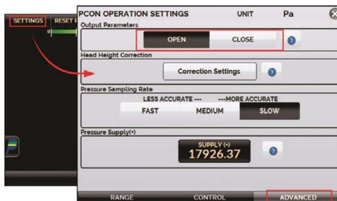
Fig. 28 - Output Isolation Valve Status
