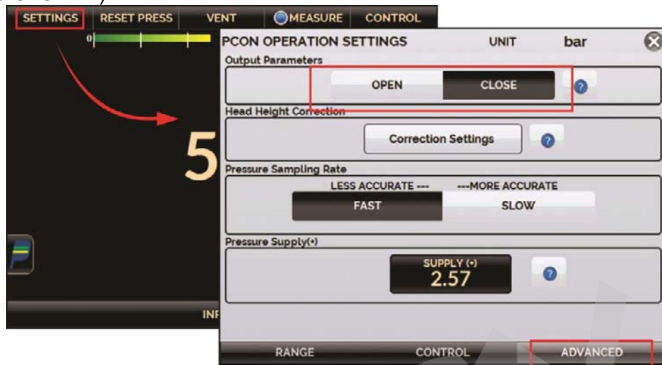
Fig. 11 - Output Isolation Valve Status
