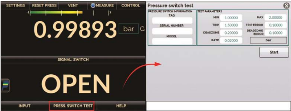
Fig. 48 - Pressure Switch Test
