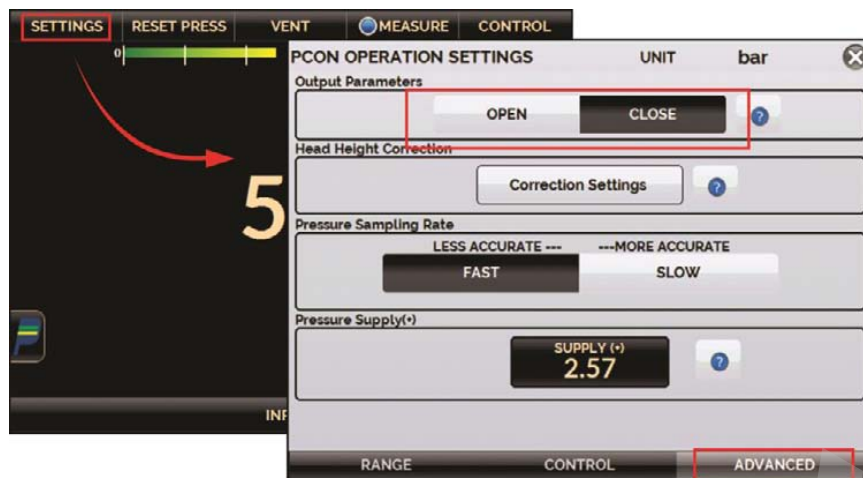
Fig. 30 - Output Isolation Valve Status
