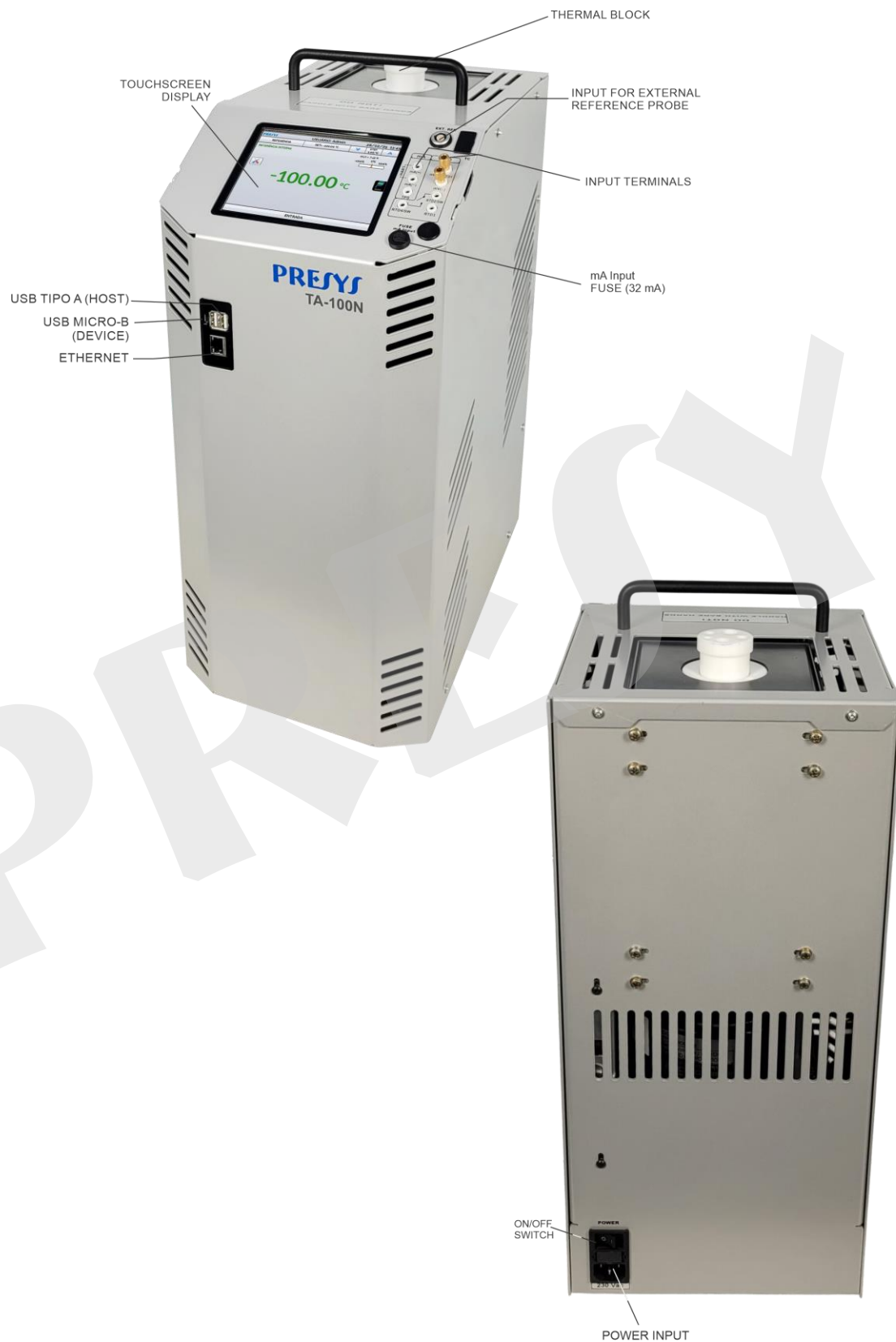
Fig. 02 - Parts Identification
