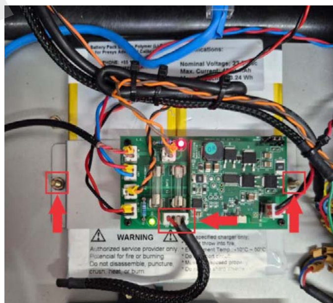
Fig. 35 - Front panel lifting and battery disconnection
