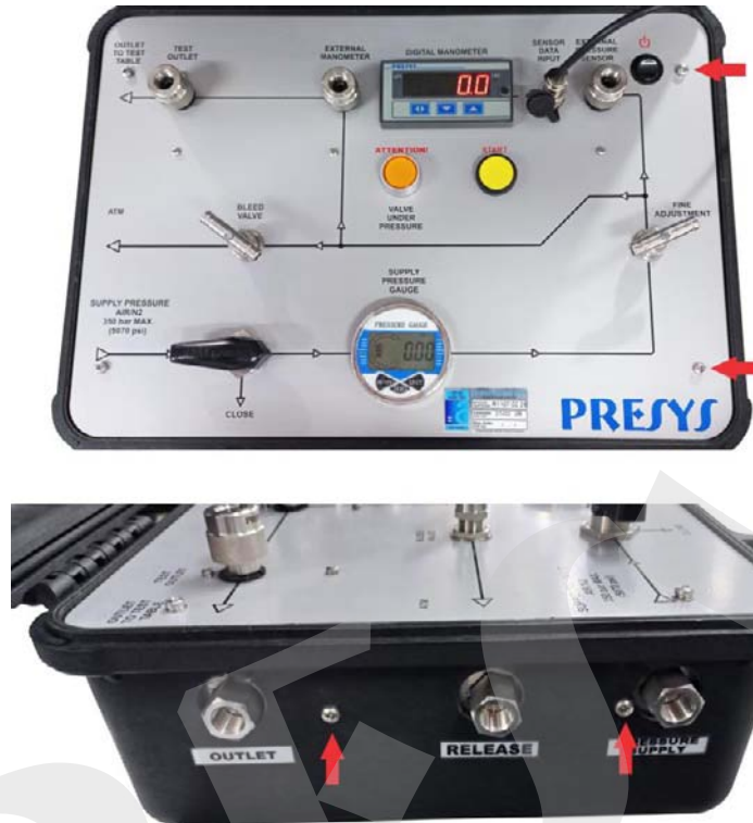
Fig. 34 - Removal of the four M4 screws
