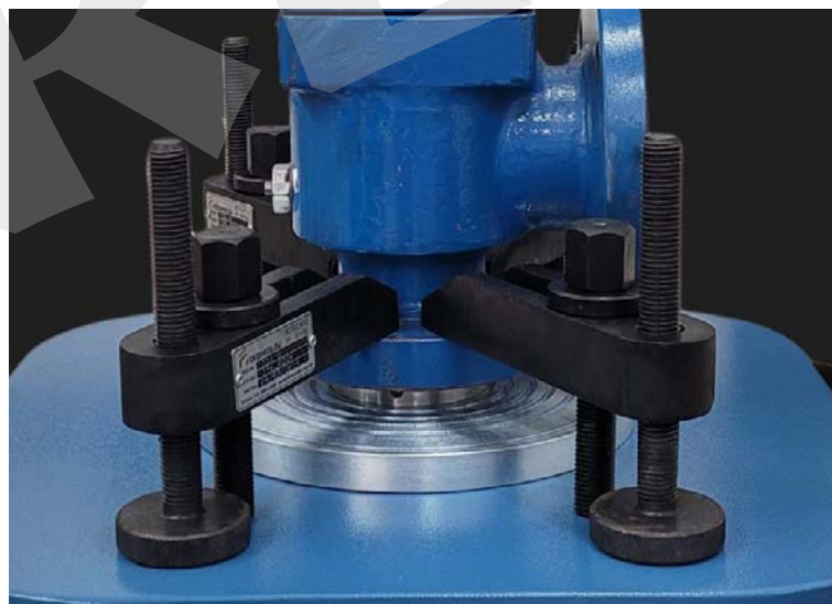
Fig.15 - Valve and centralized clamps
